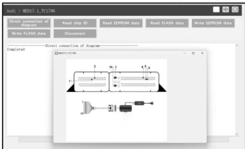
**4.1.3 Referring to the wiring diagram, use the BENCH mode cable and the corresponding adapter cable to connect the ECU and ECU&TCU programmer.**
