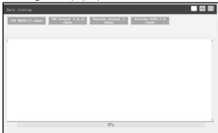
**5.2.3** Select the corresponding car model for data cloning. Follow the software prompts to load the FLASH & EEPROM data of the original vehicle ECU respectively.
